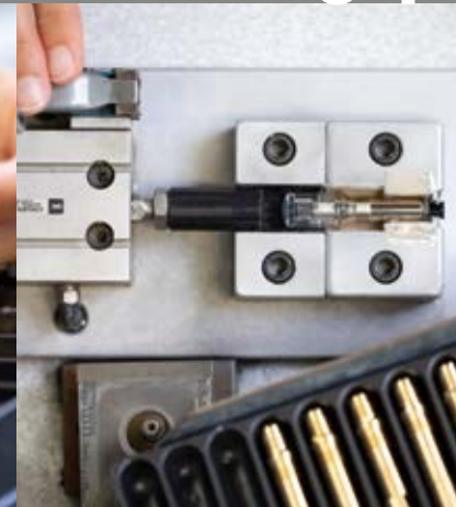
01 | Grip and spindle nut are assembled. 02 | The greased connector featuring a date stamp is screwed into the grip. 03 | Spindle and twist mechanism are assembled and are screwed into the connector. 04 | The machine uses air pressure to press the assembly together. 05 | Last of all, the piston head is placed on the spindle. The piston mechanism is now complete.
