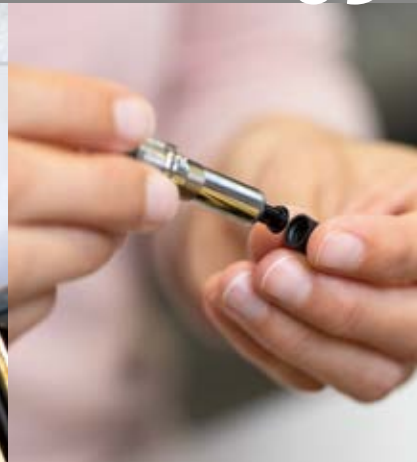
01 | Grip and spindle nut are assembled. 02 | The greased connector featuring a date stamp is screwed into the grip. 03 | Spindle and twist mechanism are assembled and are screwed into the connector. 04 | The machine uses air pressure to press the assembly together. 05 | Last of all, the piston head is placed on the spindle. The piston mechanism is now complete.
