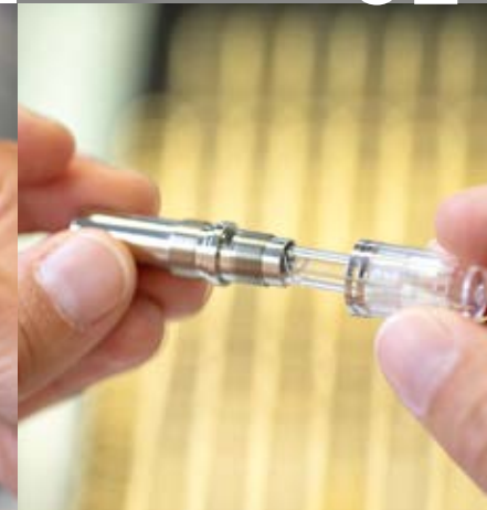
01 | Grip and spindle nut are assembled. 02 | The greased connector featuring a date stamp is screwed into the grip. 03 | Spindle and twist mechanism are assembled and are screwed into the connector. 04 | The machine uses air pressure to press the assembly together. 05 | Last of all, the piston head is placed on the spindle. The piston mechanism is now complete.
