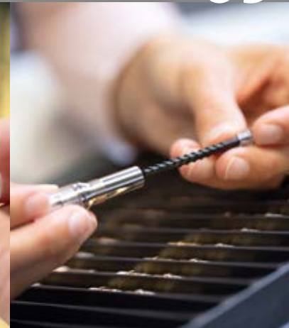
01 | Grip and spindle nut are assembled. 02 | The greased connector featuring a date stamp is screwed into the grip. 03 | Spindle and twist mechanism are assembled and are screwed into the connector. 04 | The machine uses air pressure to press the assembly together. 05 | Last of all, the piston head is placed on the spindle. The piston mechanism is now complete.
